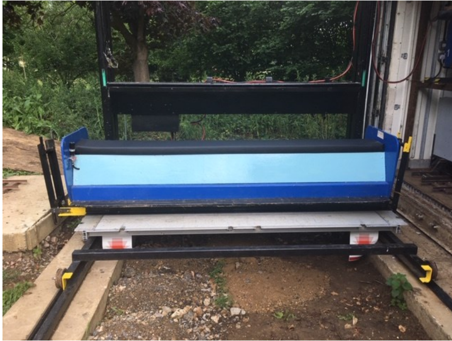
CARRIAGE RETAINED BETWEEN LOCKED HINGED LINK RAIL PRIOR TO ANY GROUND LEVEL TRAVERSE MOVEMENT
