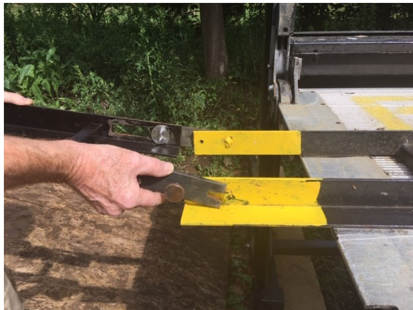
ALIGNING THE DETACHABLE HINGED LINK RAIL
