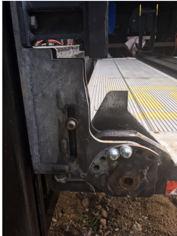
RELEASE BOLT FOR PLATFORM (RAISE AND HOLD BOLT VERTICALLY WHILST LOWERING PLATFORM)
